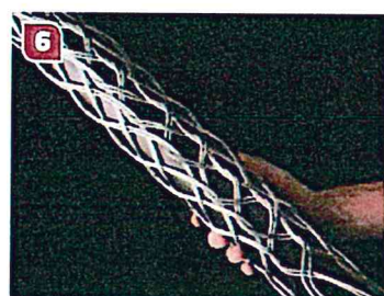
6 Try to achieve an even and neat lace-up as this assists with the strength of the stocking when pulling.
